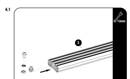
Insert two Button Head Bolts, M8 Half Nuts and M8 Schnorr Washers assemblies into the Narrow Slat as shown. Slide them to the center of the Narrow Slat (item 3), making sure that the Schnorr Washer is above the T-Slot Channel.
