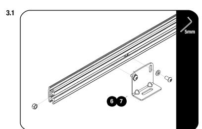
Loosely assemble the Toyota HiAce Feet (Item 6 & 7) using M8 x 16 Button Head Bolts, M8 Flat Washers and M8 Nyloc Nuts and slide them into the side profiles. They must still slide freely.
