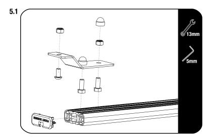
Loosely assemble the Slat Z Brackets (Item 2) to the Narrow Slats using M8 x 20 Hex Bolts and M8 Nyloc Nuts.
