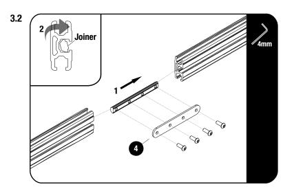
Place Joiner into the Side Profile and twist into position as shown.
