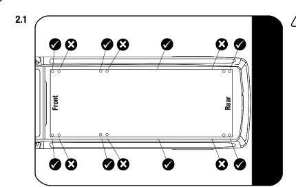
Factory Mounting Brackets to be removed. Feet will use holes as indicated. The remaining holes to be closed off with the OEM bolts supplied. Blank space indicated to be used for Mounting Foot 6.2, spaced centrally between Mounting foot 6.1 and Mounting Foot 7.
