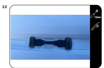
Remove Factory Mounting Bracket, use OEM mounting points to install Mounting Feet.
