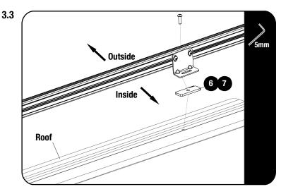
Apply Sealant around all mounting holes in the roof.
