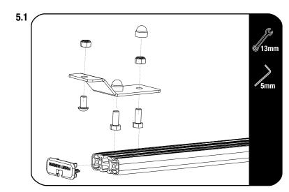
Loosely assemble the Slat Z Brackets (Item 3) to the Narrow Slats using M8 x 20 Hex Bolts and M8 Nyloc Nuts.
