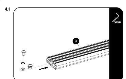
Insert two Button Head Bolts, M8 Half Nuts and M8 Schnorr Washers assemblies into the Narrow Slat as shown. Slide them to the center of the Narrow Slat (Item 3), making sure that the Scnorr Washer is above the T-Slot Channel.
