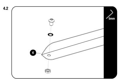
Loosely assemble the M8 x 12 Button Head Bolt, M8 Schnorr Washers and M8 Thin Nut both LH & RH Wind Deflectors (Item 4) as shown.
