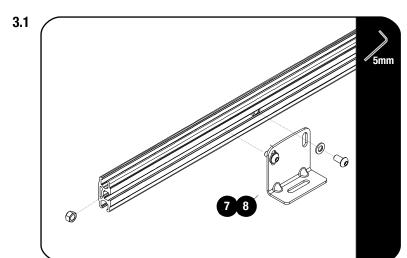
Loosely assemble the VW Crafter Feet (Item 7 & 8) using M8 x 16 Button Head Bolts, M8 Flat Washers and M8 Nyloc Nuts and slide them into the side profiles. They must still slide freely.
