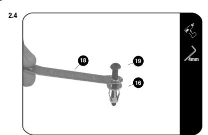
Insert a M6 x 30 Button Head Bolt (Item 19) into the Jack Nut Tool (Item 18) and loosely fit a Jack Nut (Item 16) to the button head bolt as shown.
