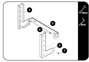
Loosely assemble the LH & RH Side Brackets (Item 3 & 4) to the Swivel Mount Bracket (Item 5) using M6 x 16 Button Head Flange Bolts and M6 Nyloc Nuts (Items 9 & 7) as shown.
