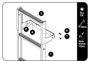
Secure the Rungs (Item 2) to the Ladder Sides (Item 1) to suit the position of the vehicle, using M6 x 25 Thread Forming Screws and M6 x 16 Flange Button Heads (Items 7 & 8). Refer to Fig 1.1.
