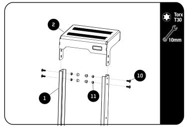
Loosely assemble the Ladder Top Bracket (Item 2) to the Ladder Side profiles (Item 1) Using M6 x 16 Flange Button Head Screws and M6 Nyloc Nuts (item 10 & 11). DO NOT FULLY TIGHTEN.
