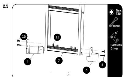
Assemble the bottom ladder Rung (Item 7) together with the two bottom mounting brackets (Item 4 & 6) to the Ladder side Profile using M6 x 25 Thread forming screws (Item 8) and M6 x 16 Button Head screws and M6 Nyloc Nuts (Item 10 & 11) as shown.
