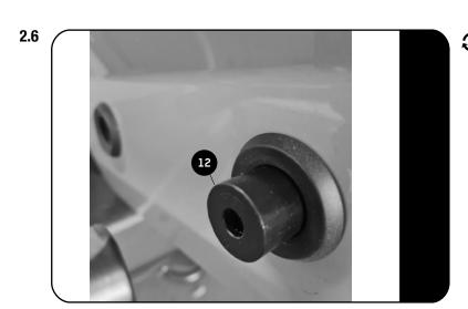
Slide the six Crush Bush assemblies (Item12) into the six cavities in the rear door as shown.
