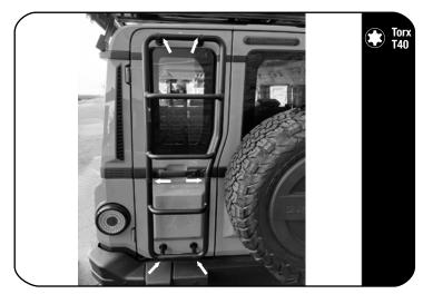
If the Vehicle has an OEM ladder fitted-Remove the 6 rubber gromets as indicated, from the ladder.
