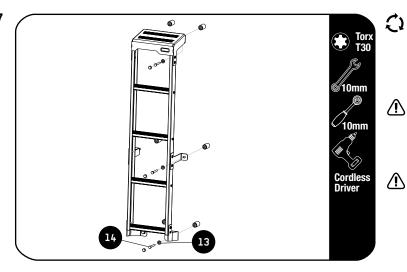
Fit the assembled Ladder to the Crush Bush Assembly fitted in 2.6 using M8 x 60 Hex Bolts and M8 x 19 x 3 Flat Washers (Item 13 & 14). Fully Tighten the M8 x 60 Hex Bolts. Fully Tighten all the M6 x 16 Button Head Screws that was loosely assembled.
