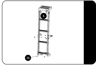
Place the M6 Nut caps (Item 5) over all the M6 Nyloc Nuts as shown. Place the M8 Nut caps (Item 15) over all the M8 Hex bolts as shown.
