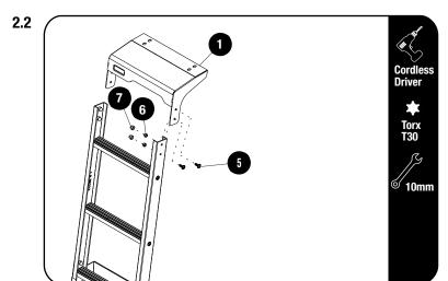
Assembly the Ladder Top (Item 1) to the parts assembled in step 2.1 using M6 x 16 Flanged Button Head Bolts (Item 5) and M6 Nyloc Nut (Item 6) and fully tighten the top and place the M6 Nut Caps (Item 7) over the M6 Nyloc Nuts.
