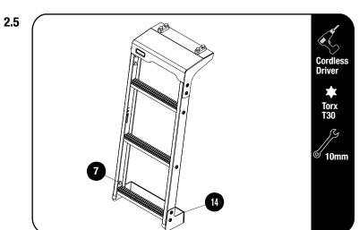
Remove the film over the VHB tape (Item 14) and stick it to your vehicle then fully tighten the Bottom Bracket (Item 13) and place the M6 Nut Caps (Item 7) over the 4 M6 Nyloc Nuts.
