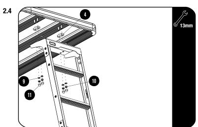
Loosely assembly the Jeep JK Side Mount Ladder to your Front Runner Roof Rack by using the 10mm HDPE Spacer (Item 4), M8 x 16 x 1.6 Flat Washer (Item 9) and the M8 Nyloc Nuts (Item 10) and fully tighten while pulling the Ladder away from the foot rail on your vehicle. When fully tightened place the M8 Nut Cap (Item 11) over all the M8 Nyloc Nuts.
