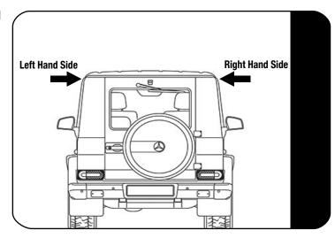
The side the door opens will determine which side the ladder will be installed.
