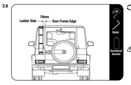
Swing open the Gutter Clamp on the top assembly. Fit the top assembly into vehicle's gutter and let the Bottom Support rest against the vehicle. Align and space the Ladder Side at the top and the Ladder Side at the bottom, 70mm away from door frame edge.
