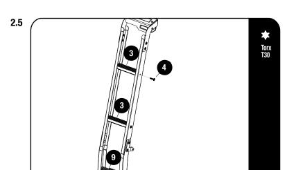
Use a little petroleum jelly on screw threads before inserting. Note these are Thread Forming Screws.
