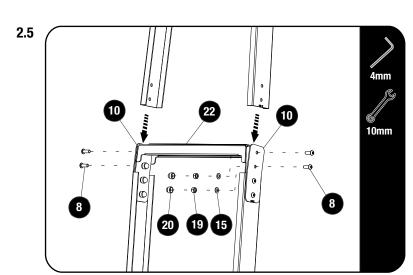
Join the top and bottom assemblies by sliding the top ladder assembly between the Joiner Plates (Item 10) and the Ladder Rung (Item 22).
