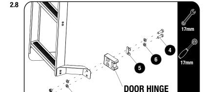
Loosely secure the Ladder to the hinge outer casting at the top of the door using two M10x30 Hex Head Bolts, four M10 Flat Washers, one Washer Plate and two M10 Nyloc Nuts (Items 4, 6, 5 & 9).
