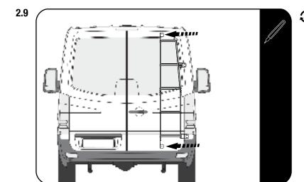
Mark the left-hand side top & bottom holes on the door as shown.
