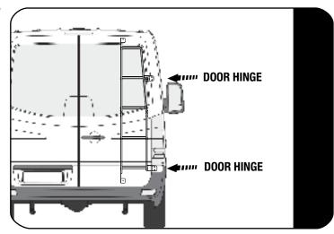
Working on the right rear door, open the door and have a friend position the Ladder so that the mounting holes align with the existing holes in the top and bottom door hinge outer castings as shown in 2.8.
