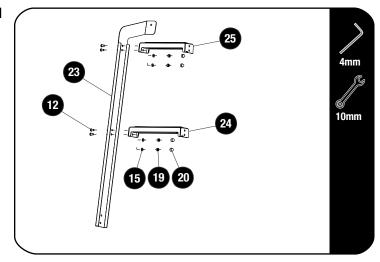
Assemble the Ladder Rung (Item 25) and the Ladder Rung (Item 24) to the Top LH Ladder Side (Item 23) using four M6x12 Button Head Screws, four M6 Flat Washers and four M6 Nyloc Nuts (Item 12, 15 & 19). Finish off by placing six M6 Nut Caps (Item 20) on the M6 Nyloc Nuts.
