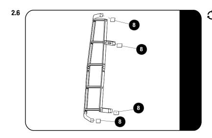
Remove backing and place the four Foam Rubber Pads (Item 7) onto the ladder's feet and trim to fit.
