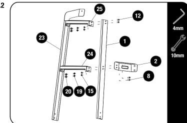
Assemble the Top RH Ladder Side (Item 1) and the Top Hinge Bracket (Item 2) to the assembly in 2.1, using two M6x12 Button Head Screws, two M6x16 Button Head Screws, four M6 Flat Washers and four M6 Nyloc Nuts (Item 12, 8, 15 & 19). Finish off by placing four M6 Nut Caps (Item 20) on the M6 Nyloc Nuts.
