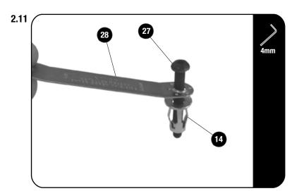
Insert the M6 x 25 Button Head Bolt (Item 27) into the one side of the M6 Jack Nut Tool (Item 28). Loosely fit a M6 Jack Nut (Item 14) to the Button Head Bolt as shown.
