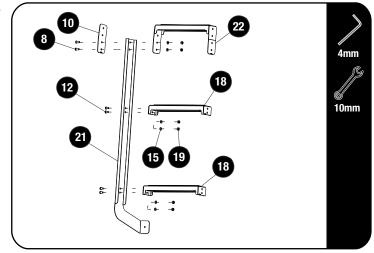
Assemble the two Ladder Rungs (Item 18) to the Bottom LH Ladder Side (Item 21) using four M6x12 Button Head Screws, four M6 Flat Washers and four M6 Nyloc Nuts (Item 12, 15 & 19).
