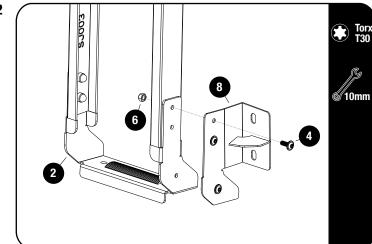
Loosely assemble the Bottom Mount Bracket and Ladder Hinge Bracket (Item 2 & 8) to the assembly in 2.1 using M6 x 16 Flange Button Head Bolts and M6 Nyloc Nuts (Items 4 & 6).
