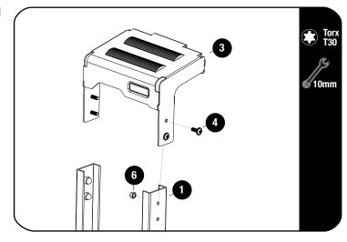
Loosely assemble the Ladder Rung
