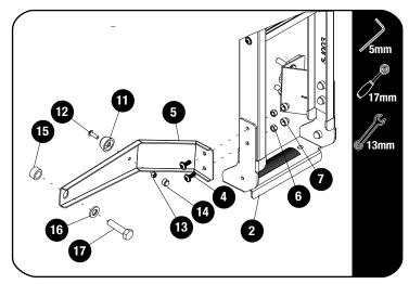
Assemble the Spare Wheel Mounting Bracket (Item 5), by attaching the Buffer (Item 11) with the M5 x 16 Button Head Bolt, M5 Nyloc Nut and M5 Nut Cap. (Items 12,13 and 14).
