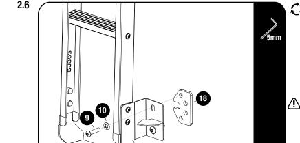
Secure the Ladder Hinge Mount Bracket to the hinge using M8 x 35 Button Head Bolts, M8 x 16 x 1.6 Flat Washers and the Hinge Spacer (Items 9, 10 & 18)
