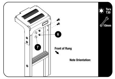
Fully tighten all Fasteners.
