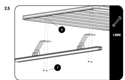
Loosely fit your Slimline II Rack by using M8 x 25 Hex Bolts and M8 Nylocs (Items 7 and 9) as shown.
