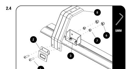
Assemble the Legs (Item 8) to the Leg Mount (Item 3) by using M8 x 25 Button Heads and M8 nyloc Nuts (Items 4 & 7)
