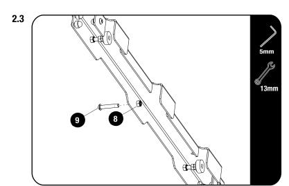
Secure three M8 x 50 Hex Bolts (Item 9) to each Side Rial (Item 1) using M8 Nyloc Nuts (Item 8) as shown.
