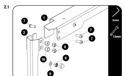
Assemble The Bottom Side Rails (Item 1) to the Front and Rear Legs (Item 2) as shown using the M8 x 12 Button Head Bolts M8 Nyloc Nut and M8 Nut Cap (Item 6,7 & 8).
