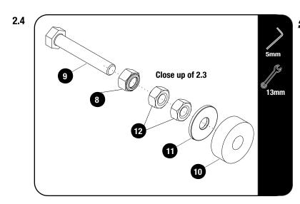
From the inside of the side rail, assemble two M8 Plain Nuts followed by one M8 x25 x2 Flat Washer and one 10mm Spacer (Item 10, 11 & 12) to the M8 x 50 Hex Bolts secured in 2.3.
