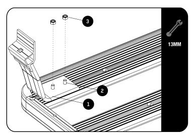
C1 Loosely fit the Legs (Item 1) using M8 Nyloc Nuts (Items 2 & 3)
