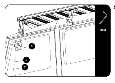
Secure the Gutter Clamps (Item 5) using M8 x 30 Button Heads and M8 Schnorr Washers (Items 6 & 7).
