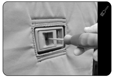
Open the vehicle left hand rear door. Loosen and remove the screw securing the latch to the inside of the rear door using a Phillips Screw Driver.
