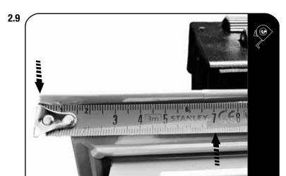
Position the Ladder 70mm from the top door edge as shown.
