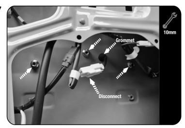
Peel back the plastic cover to expose the wiring and door fasteners.
