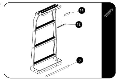
Remove the backing tape of the two Rubber Protective Strips (Item 3) and secure the strips to the Support Bracket as shown.
