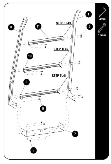
Loosely assemble the LH Ladder Side (Item 8) and the RH Ladder Side (Item 1) to Ladder Rungs (Item 9, 10 & 11) and the Bottom Support (Item 7) using M6x12 Button Head Screws & M6 Nyloc Nuts (Items 2 & 5).
