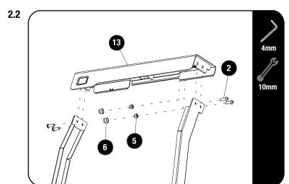
Fully assemble the Ladder Top Step (Item 13) to the assembly.
