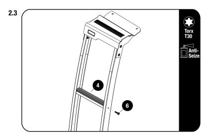
Apply a little Anti seize/oil on screw threads before inserting.
