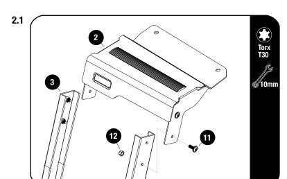
Loosly assemble the Top Step (Item 2) to the Ladder Sides (Item 3) using M6 x 16 Flange Button Head Bols and M6 Nyloc Nuts (Items 11 & 12).
