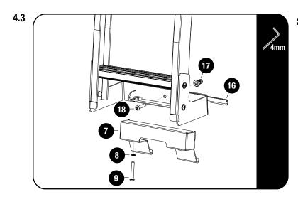
Secure the Ladder to the rear hatch using a M6 x 25 Button Head Bolt (Item 18).
