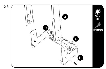
Loosly assemble the Bottom Bracket (Item 5) to the Ladder Sides (Item 3) using M6 x 16 Flange Button Head Bols and M6 Nyloc Nuts (Items 11 & 12).
