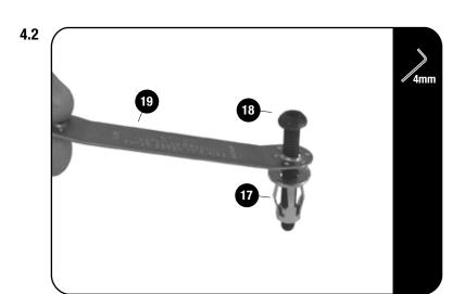
Insert a M6 x 25 Button Head Bolt (Item 18) into the Jack Nut Tool (Item 17) and loosely fit a Jack Nut (Item 19) to the button head bolt as shown.
