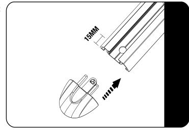
Should you wish to fit the End Caps to the Rail, you will need to drill a 8.5 mm Hole 15mm in from each end as shown. Only fit the End Caps once the Tie Down Rail has been fitted to the vehicle and the Channel Nut has been inserted.
