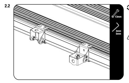
Fasten all bolts securely using a 5mm Hex key and 13mm wrench.
