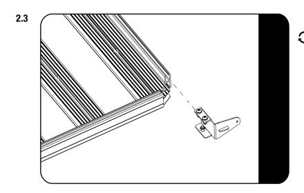
Slide the LH and RH Front Mount Brackets into the Profile.
