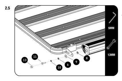
Secure the light bar to the Mounting
