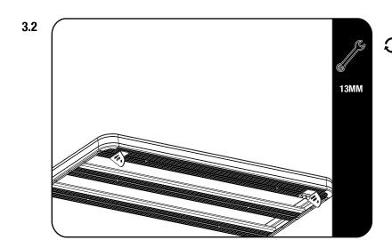
Using a tape measure, space the Brackets accordingly to suite the length of the light bar you will be fitting.
