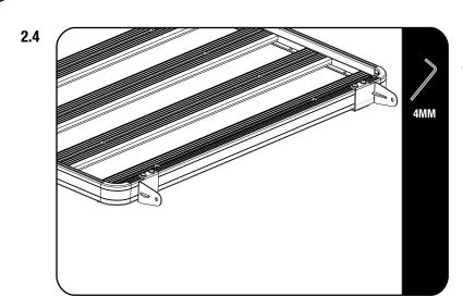
Using a tape measure, space the Brackets accordingly to suite the length of the light bar you will be fitting.
