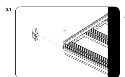
Remove the front right hand side corner piece.
