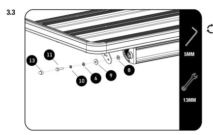
Secure the light bar to the Mounting Brackets using two M8 x 25 Hex Bolts, two M8 Spring Washers, two M8 x 16 x 1.6SS Flat Washers, the Spacer and M8 x 19 x 2SS Flat Washers (Items 11, 10, 6, 9 & 8) as shown
