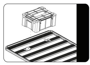
Use the T-Slot Rubber (Item 5) included and insert into the T-Slot to help prevent cargo from moving and to protect your rack.
