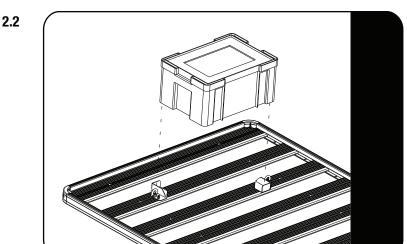
Use the T-Slot Rubber (Item 5) included and insert into the T-Slot to help prevent cargo from moving and to protect your rack.
