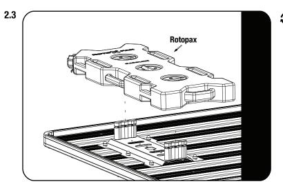
Place the Rotopax tank over the RotoPax RX-PM Pack mounts and tighten.
