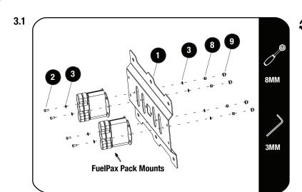
Fit two FuelPax Mounts to the Rotopax Mounting Plate (Item1) using four M5 x 12 Button head, eight M5 Flat Washers and four M5 Nyloc Nuts (Item 2,3 and 8). Finish it off by placing an M5 Nut Cap (Item 9) over each M5 Nyloc Nut (Item 8).
