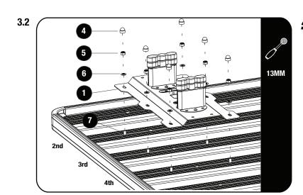
Slide two M8x16 Hex Bolts (Item 7) into each of the 2nd, 3rd and 4th slats t-slot. Place the Rotopax Mounting Plate (Item 1) over the bolts. Move the Mounting Plate into the desired position by using the Fuelpax tank before securing it with M8 Nyloc Nut and M8 Flat Washer (Item 5 & 6). Finish it off by placing an M8 Nut Cap (Item 4) over each M8 Nyloc Nuts (item 5).
