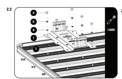
Slide two M8x16 Hex Bolts (item 7) into each of the 2nd, 3rd and 4th slats t-slot. Place the Rotopax Mounting Plate (Item 1) over the bolts. Move the Mounting Plate into the desired position by using the Rotopax tank before securing it with M8 Nyloc Nut and M8 Flat Washer (Item 5 & 6). Finish it off by placing an M8 nut cap (Item 4) over each M8 Nyloc Nuts (Item 5).
