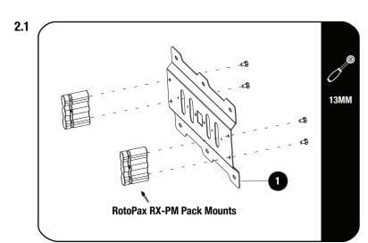
Fit two RotoPax RX-PM Pack Mounts to the Rotopax Mounting Plate (item1). Fasteners are supplied with the RotoPax RX-PM Pack Mounts.
