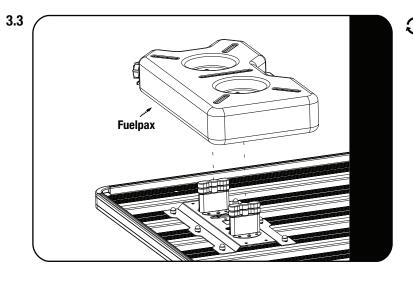
Place the Fuelpax tank over the FuelPax Mounts and tighten.
