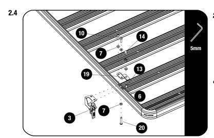
Place the Rack Mount Brackets (Item 3) over the side profile, followed be the Rack Support (Item 19) and secure using M8 x 25 Button Head Bolts, M8 x 30 Button Head Bolts, M8 x 16 Hex Bolts, M8 x 16 x 1.6 Flat Washers and M8 Nyloc Nuts (Items 6, 7, 10, 13 & 20) as shown.
