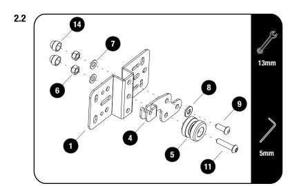
Assemble the Bobbins and Catches (Items 4 & 5) to the Awning Mount Brackets (Item 1) using a M8 x 20 Button Head Bolts, M8 x 35 Button Head Bolts, M8 x 19 x 2 Flat Washers, M8 x 16 x 1.6 Flat Washers and M8 Nyloc Nuts (Items 6, 7, 8, 9 & 11) as shown.
