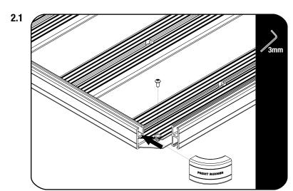
Choose where you would like to mount your Light bracket. Remove the Corner from the Rack and Slide the M8 Nyloc Nut (Item 4) into the Side Profiles T-Slot.
