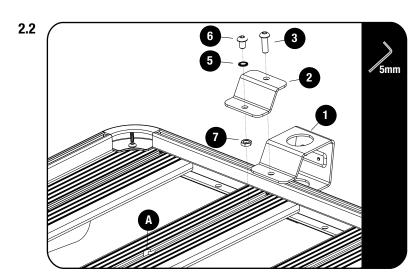
Secure the Light Bracket and the Rack Support Bracket (Item 1 & 2) to the Rack using M8 x 25 Button Head Bolt, M8 Nyloc Nut, M8 Schnorr Washer, M8 x 12 Button Head Bolt and a M8 Thin Nut, inserted via the slat pocket as indicated by (A) (Items 3, 4, 5, 6 & 7).
