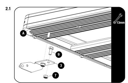
Loosly assemble the Under Rack Mounting Bracket (Item 3) to the front combined slat as shown using M8 x 16 Hex Head Bolts and M8 Nyloc Nuts (Items 7 & 9).
