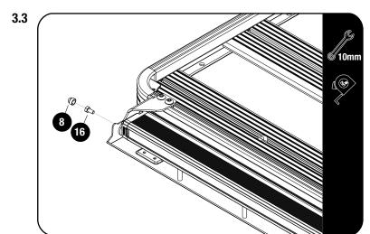
Loosly assemble the Light Bar (Sold Separately - LIGH213) to assembly 3.2 using M6 x 12 Hex Bolt. Center the Brackets and fully tighten all fasteners.
