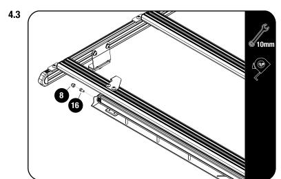
Cosly assemble the Light Bar (Sold Separately - LIGH213) to assembly 4.2 using M6 x 12 Hex Bolt. Center the Brackets and fully tighten all fasteners.
