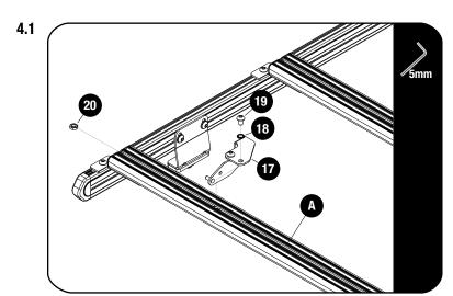
Loosly assemble the Van Rack Mounting Bracket (Item 17) to the front slat as shown using M8 x 12 Button Head Bolts, M8 Schnorr Washers and M8 Half Nuts (Items 18, 19 & 20).
