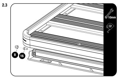
Loosly assemble the Light Bar (Sold Separately - LIGH213) to assembly 2.2 using M6 x 12 Hex Bolt. Center the Brackets and fully tighten all fasteners.
