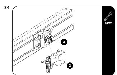
Slide the Rack Mount Bracket (item 2) onto the Bobbin Assembly.
