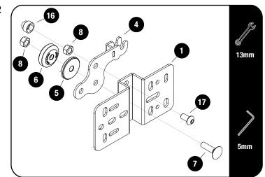
Assemble the Catch, Male Bobbin & Female Bobbin (Items 4, 5 & 6) to the Awning Bracket (Item 1) using M8 x 30 Carriage Bolt and a M8 Nyloc Nut (Items 7 & 8), do not fully tighten.
