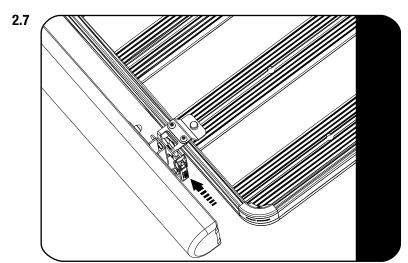
Position the assembled awning over the Rack Brackets and slot down into position.
