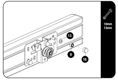
Loosely fit the assembly from 2.2 onto the back of your awning. Depending on the make of your awning use either M6 x 16 or M8 x 16 Hex Bolts, Nyloc Nut and Flat Washers. (Items 8, 10, & 13 or 11, 12 & 14) as shown
