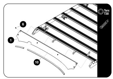
Fit the Wind Fairing Rubber (Item 10) to the Light Bar Wind Fairing (Item 1). Using the notched section as a guide, trim if needed.
