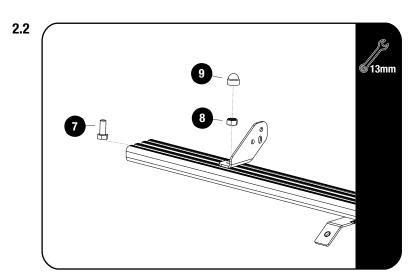
Fit the Light Bar Bracket 01 LH / RH (Item 4) for for the 40" Light Bar, using M8 x 16 Hex Bolts & M8 Nyloc Nuts (Items 7 & 8). Fit the light bar and center it on the slat before fully tightening the brackets.
