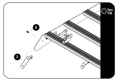
Secure the Wind Fairing Side Supports LH / RH (Item 2) to the foot rails bottom holes as shown using M6 x 16 Flange Button Head (Item 6).
