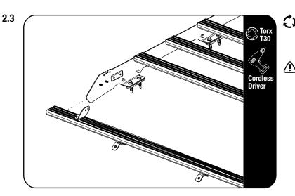
Secure assembly 2.2 to the front two top holes on the foot rails using the fasteners supplied with KSFF001.
