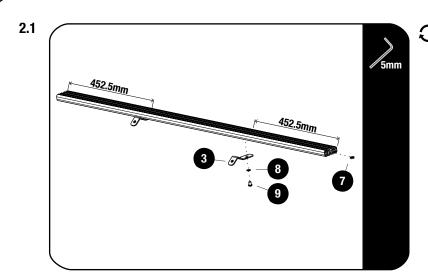
Measure 452.5mm inward from both ends of the slat and center both Mid Support Brackets on these points. secure using a Schnorr Washer and M8x12 Button Head (Items 8 & 9). Fully tighten.
