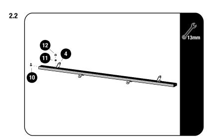
Fit the Light Bar Bracket 01 (Item 4) for for frontrunner 40" light bar, using M8x16 Hex Bolt & M8 Nyloc Nut (Items 10 & 11). Fit light bar and center on slat before fully tightening the brackets.
