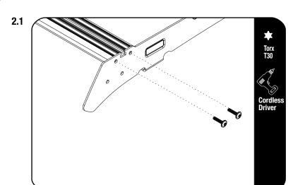
Start by undoing the bolts on the front of the Roof rack holding the front slat inplace using a T30 Torque bit.
