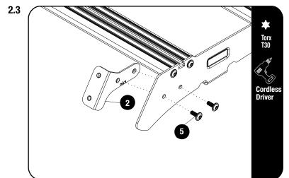
Assemble the Wind Fairing Outer Support Bracket (Item 2) Left and Right side with the M6 x 16 Button Head Flange Bolt (Item 5) as shown.
