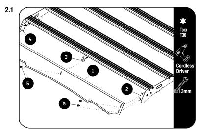
Assemble the Wind Fairing (Item 1) to the Support Brackets (Item 2 , 3 & 4) useing the M6 x 16 Button Head Flange Bolts using a T30 Torx as shwon.
