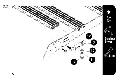
$\mbox{\it C1}$  Slide the M8 x 20 Hex Bolt (Item 12) into the slat as shown.
