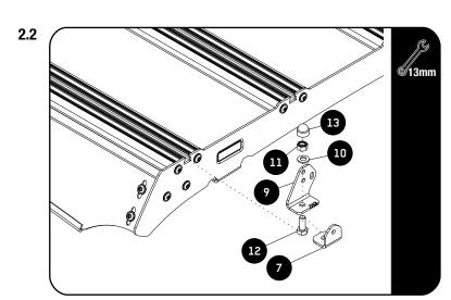
If you would want to fit a Light Bar with the Wind Fairing Slide the M8 x 20 Hex bolt (Item 12) into the Front Slat that was removed in 2.1 as shown, with the Light Bar Bracket (Item 7) assembeld togheter with the M8 Flat Washer and M8 Nyloc Nut (Item 10 & 11) as shown and fully tighten.
