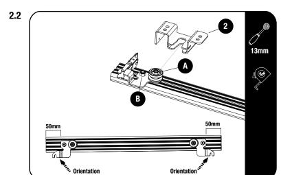
Slide the Latch Plate (Item 2) onto the Bobbin Assembly.
