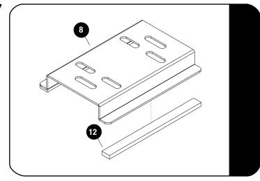
Remove the backing tape of the Self Adhesive Rubber Strips (Item 12) and secure it to the four Box Brackets (Item 8).
