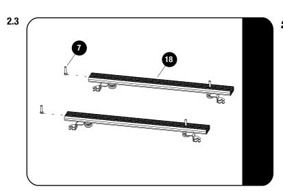
Turn the assembled slats over and slide four M8x45 Hex Head Bolts (Item 7) into the assembled slats as shown.
