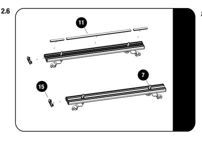
Insert the T-Slot Rubbers (Item 11) into the T-slot of each Slat with the M8x45 Hex Head Bolts (Item 7) positioned as shown.
