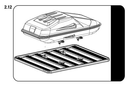
Lower the Cargo Box onto the rack making sure the Quick Release Feet align with the rack mounted Catch Brackets.
