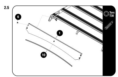
Fit the Wind Fairing Rubber (Item 10) to the Wind Fairing (Item 1). Using the notched section as a guide, trim if needed.
