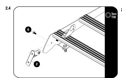
Secure the Wind Fairing Side supports LH / RH (Item 2) to the foot rails bottom holes as shown using M6 x 16 Flange Button Heads (Item 6).
