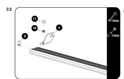
Fit the Light Bar Bracket 01 LH / RH (Item 4) for for the 40" Light Bar, using M8 x 16 Hex Bolt & M8 Nyloc Nut (Items 9 & 10). Fit the light bar and center it on the slat before fully tightening the brackets.
