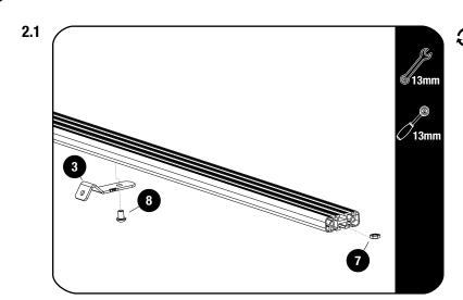
Slide one M8 Thin Nut (Item 7) into the T-Slot of the front slat. Center the Mid Support Bracket (Item 3) in the Middle of the slat and secure using a Button Head Bolt (Item 8). Fully tighten.
