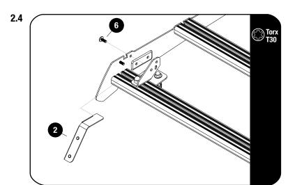
Secure the Wind Fairing Side supports LH / RH (Item 2) to the foot rails top holes as shown using M6 x 16 Flange Button Heads (Item 6).
