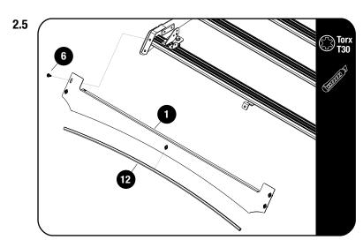
Fit the Wind Fairing Rubber (Item 12) to the Light Bar Wind Fairing (Item 1). Using the notched section as a guide, trim if needed.
