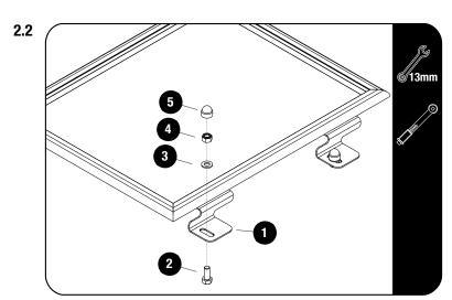
Determine which slats you will be using to mount your Zamp Solar panel and Slide the M8 x 20 Hex Head Bolts into the machined pockets in the slats. Secure the assembly from 2.1 using M8 x 20 Hex Head Bolts, M8 x 16 x 1.6 Flat Washers and M8 Nyloc Nuts (Item 2, 3 & 4). Fully Tighten.
