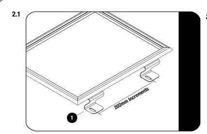
Slide the T-nut into the solar panel frame, refer to the Zamp Solar Fitment guide. Loosly assemble the Bracket (Item 1) to the frame using the fasteners supplied with the Zamp Solar Panel Kit. Space the Brackets at 202mm increments and fully tighten.
