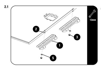
Loosely assemble the Universal Solar Panel Mounting Brackets (Item 1) to your solar panel using M8 x 16 Hex Bolts, the M8 x 16 Washers and M8 Nylock Nuts (Items 2, 3 & 5)
