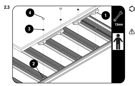
Slide the M8 x 16 Hex Bolts (Item 2) into the slats machined slots to the corresponding slats. Fasten the the Universal Mounting Bracket (Item 1) to the slats with the M8 Hex Nuts (Item 3).
