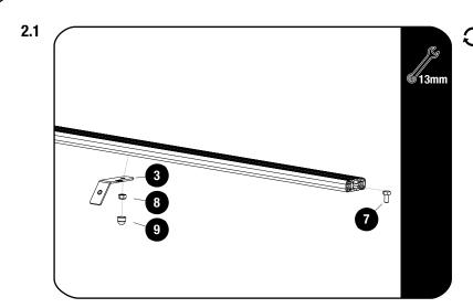
Slide one M8 x 16 Hex Head Bolt (Item 7) into the T-slot of the front slat. Center the mid support bracket in the middle of the slat and secure using M8 Nyloc Nut (Item 8). Fully tighten.
