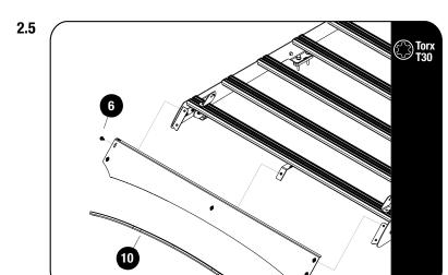
Fit the Wind Fairing Rubber (Item 10) to the Light Bar Wind Fairing (Item 1). Using the notched section as a guide, trim if needed.
