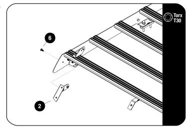
Secure the Wind Fairing Side Supports LH / RH (Item 2) to the foot rails top holes as shown using M6x16 Flange Button Head
