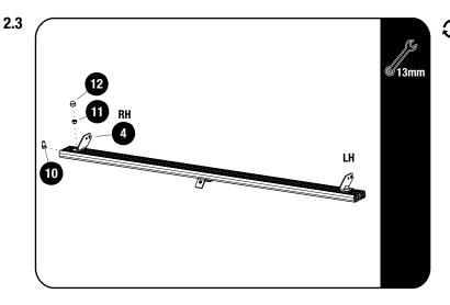
Fit Light Bar Bracket 01 LH / RH (Item 4) for for Front Runner 40" light bar, using M8x16 Hex Bolt & M8 Nyloc Nut (Items 10 & 11). Fit light bar and center on slat before fully tightening the brackets.
