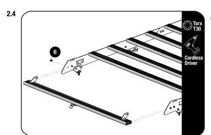
Secure assembly 2.3 to the front two bottom holes on the foot rails using the M6 x 16 Flange Button Head (Item 6). Fully tighten.
