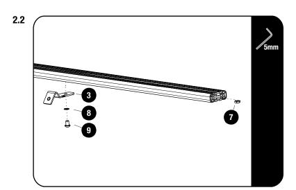
Remove the wind fairing mid support bracket that is currently on the slat and replace it with the fairing mid support bracket supplied with this kit (Item 3).
