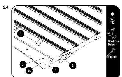
Assemble the Wind Fairing and Wind Fairing Rubber Seal (Item 2 & 10)
