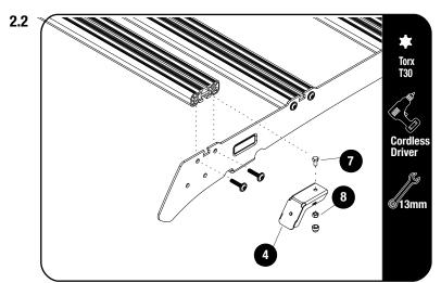
Slide the M8 x 16 Hex Bolt (Item 7) into the slat as shown.
