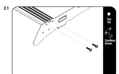
Start by undoing the bolts on the front of the Roof rack holding the front slat inplace using a T30 Torque bit.
