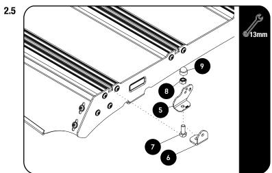
If you would want to fit a Light Bar with the Wind Fairing Slide the M8 x 20 Hex bolt (Item 7) into the Front Slat that was removed in 2.1 as shown, with the Light Bar Bracket 01 (Item 5) assembled together with the M8 Nyloc Nut (Item 8) as shown and fully tighten.
