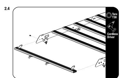
Secure assembly 2.3 to the front two bottom holes on the foot rails using the fasteners removed in step 2.1. Fully tighten.
