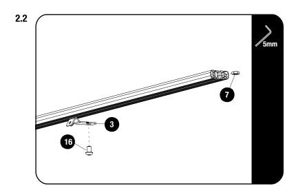
Remove the Wind Fairing Centre Support Bracket that is currently on the slat and replace it with the Wind Fairing Centre Support Brackets supplied with this kit (Item 3).
