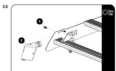
Secure the Wind Fairing Side Supports LH / RH (Item 2) to the foot rails top holes as shown using M6 x 16 Flange Button Head Bolt (Item 4).
