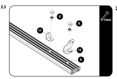
Use the Light Bar Bracket High profile (Item 12) to fit a high profile Light Bar.
