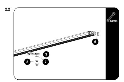
Remove the Wind Fairing Centre Support Bracket that is currently on the slat and replace it with the Wind Fairing Centre Support Bracket supplied with this kit (Item 3).
