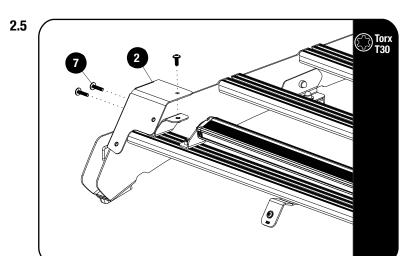
Use the Wind Fairing Side Supports LH / RH (Item 2) to space the Inner Support installed in step 2.4 and the fully tighten the Inner Supports.
