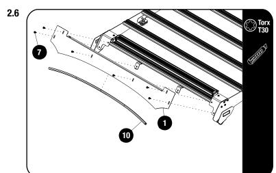
Fit the Wind Fairing Rubber (Item 10) to the Light Bar Wind Fairing (Item 1). Using the notched section as a guide, trim if needed.
