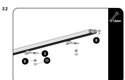
Slide two M8 x 16 Hex Head Bolts (Item 8) into the bottom T-slot of the front slat. Position the Center Support Brackets (Item 3) at equal distances from the middle of the slat using the Wind Fairing as a guide for the two positions, and secure using a M8 Nyloc Nut (Item 9).
