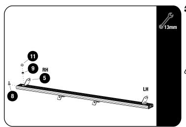
Fit Light Bar High Profile Bracket LH / RH (Item 5) for the Front Runner 40" light bar, using M8 x 16 Hex Bolt & M8 Nyloc Nut (Items 8 & 9). Fit the light bar and center on the slat before fully tightening the brackets.
