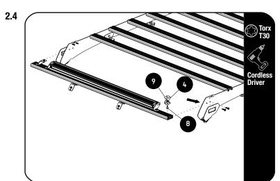
Loosely fit the Inner Supports (Item 4) using M8 x 16 Hex Head Bolts (Item 8) and M8 Nyloc Nuts (Item 9).
