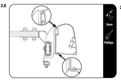
Using a 3mm drill bit, drill through the pre-drilled holes in the adapter, into and through the first skin of the awning.
