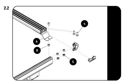
Loosen both Z brackets (Item A) of each slat chosen for the awning brackets as well as the Z brackets of each slat between the central bracket and one of the outer slats.
