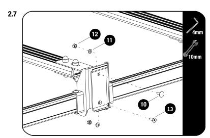
Depending on the length of your Dometic Awining, you may need either a narrow adapter or a wide adapter (shown in 2.6) mounted to the center Awning Mounting Bracket.
