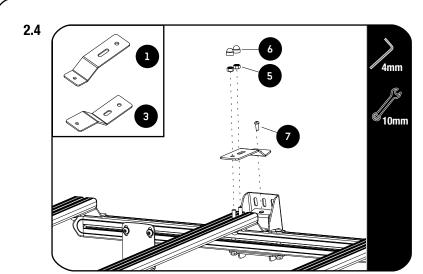
Secure the High Slat Position Support Bracket (Item 1) or Low Slat Position Support Bracket (Item 3) to the Awning Mounting Bracket (Item 2) using one M6 x 16 Button Head Bolt (Item 7).
