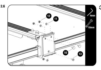
Secure the adapter (supplied with the awning) to the Awning Mounting Bracket using M6 x 16 Square Neck Bolts, M6 x 16 Countersink Socket Screw, M6 x 12 x 1 Flat Washer and M6 Nyloc Nuts (Items 10, 13, 11 and 12).
