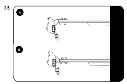
Take note which Support Bracket should be used. Item 1 as shown in step 2.4 for High/Raised Slat position (A) or Item 3 as shown in step 2.4 for Low/Inverted Slat position (B).
