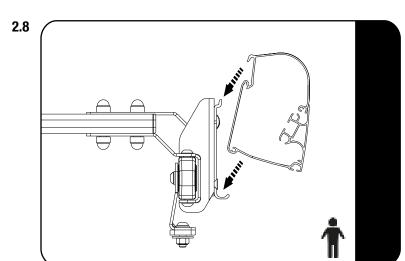
With the help of a friend, hook the awning onto the adapter as shown in step 2.6 and 2.7.
