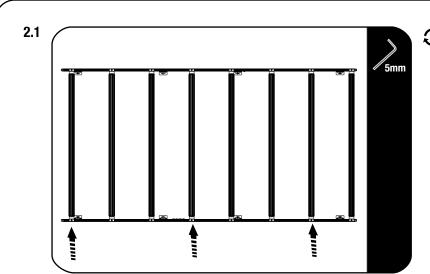
The Awning is mounted on all three brackets, two in the outer positions and the third centrally. Once you have decided on the awning's position, you need to identify the three slats that need to be used.
