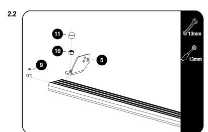
Fit the Light Bar Bracket 01 LH / RH (Item 5) for for the 40" Light Bar, using M8 x 16 Hex Bolt & M8 Nyloc Nut (Items 9 & 10). Fit the light bar and center it on the slat before fully tightening the brackets.
