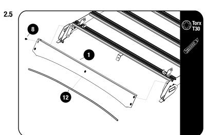
Fit the Wind Fairing Rubber (Item 12) to the Wind Fairing (Item 1). Using the notched section as a guide, trim if needed.
