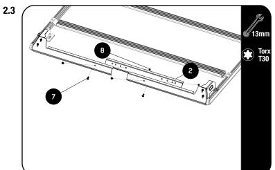
Assemble the Fairing Brace (Item 2) to the Wind fairing fitted in 2.2 using M6 x 16 Flange Button head bolts and M6 Nyloc Nuts (Item 7 & 8).
