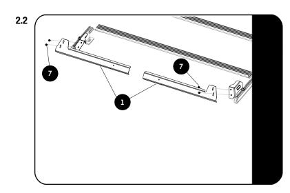
Loosely Assemble the Wind Fairing (Item 1) using the M6 x 16 Flange Button Head Screw (Item 7) as shown. Do this Both LH and RH side.DO NOT FULLY TIGHTEN.
