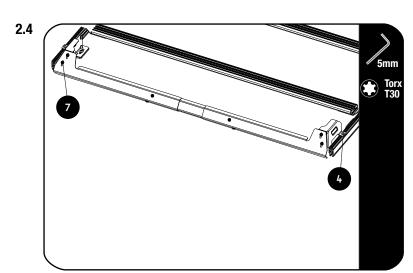
Fully Tighten the M8 x 16 Button Head Screws (Item 4) fitted in 2.1
