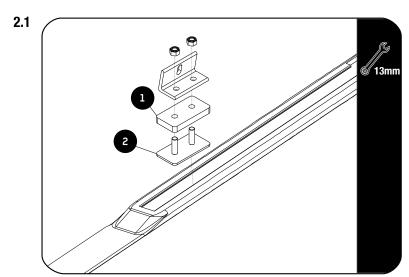
Assemble the Stud Plate and Stud Plate Spacer (Items 1 & 2) as shown. Insert the Stud Plate assemblies into the vehicle's OEM rails as shown. Do this both LH and RH side.
