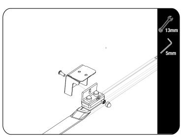
Secure the Mounting Foot to the assembly from 2.1 using the hardware supplied with FASS028.
