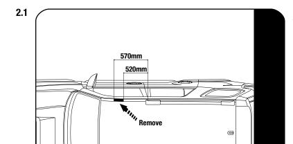
With the factory rails removed, use the center of the existing front hole of the roof rail,mark out the dimension as shown on the ditch molding. Do this on the left and right side.
