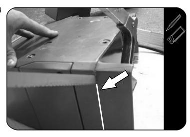
Mark and cut the rear bottom section off the center console as shown.
