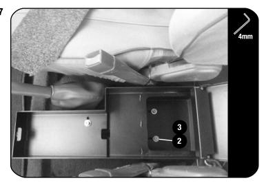
Open the Safe and console assembly, remove the interior carpet and hidden compartment cover.
