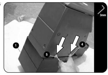
Place the center console over the Safe (Item 1) as show, lining up the holes in the side of the center console with the mounting points on the Safe.
