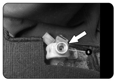
Locate the the front mounting point next to the vehicle's gear lever as indicated by the arrow and place the Aluminium Spacer (Item 6) supplied on top of the mounting point as shown.
