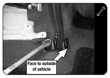
Loosen and rotate the two seat belt brackets as shown.
