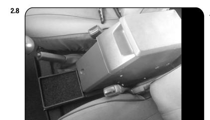
Refit the interior carpet and hidden compartment cover. Close the Safe, remove the key and place the supplied carpet over the lock and front section of the Safe as shown.
