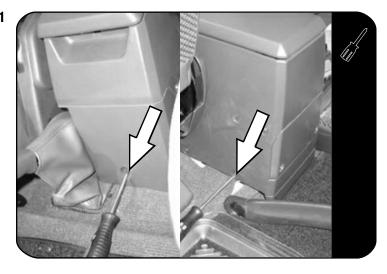
Loosen the center console found between the driver and front passenger seat by removing the three bolts as indicated, one in the front and one either side on the rear.
