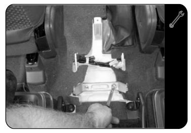
Loosen and remove the original console mounting bracket. The two mounting points will be used later to secure the Safe to the vehicle.
