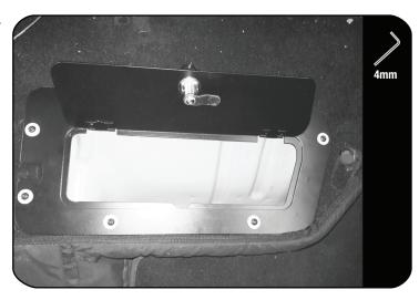
Secure the LH Safe (Item 2) over the LH compartment using five M6 x 20 Button Head Screws and five M6 Large Washers (Items 3 & 4).
