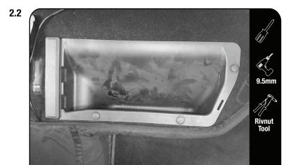
Remove the three plastic rivets from the LH compartment tray.
