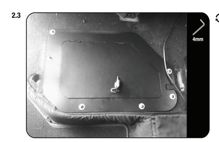
Secure the RH Safe (Item 1) over the RH compartment using six M6 x 20 Button Head Screws and six M6 Large Washers (Items 3 & 4)
