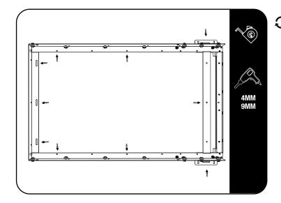
Make sure you have closed the load bed tail gate to ensure that it does not make contact with the frame. Once you are satisfied with the positioning of the frame, mark the position of all the mounting points as indicated by the arrows onto the load body.
