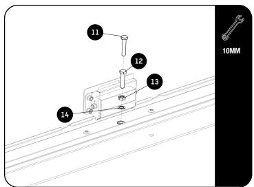
Before refitting the slide to the frame, use the M6 x 35 or M6 x 40 hex bolt (Item 11 or 12) (depending on which fits the specific vehicle best) together with the M6 Normal nut and M6 x 12 x 1 Flat washer (Item 13 & 14) and assemble as shown.
