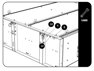
Secure four D-Rings (Item 10) on the side of the drawers pillars using M6 x 20 Hex Bolts, M6 SS Spring Washers and M6 x 19 x 1SS Flat Washers as shown.
