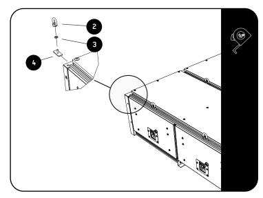
Assemble the Eye-Nuts with a M6 Nylon Washer and a Stud Plate (Items 2, 3 & 4) and slide them into the extrusion.
