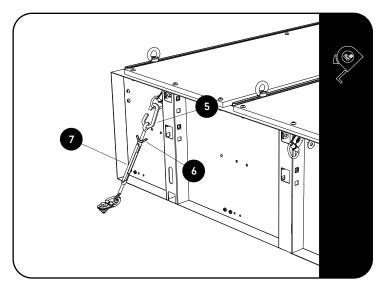
Attach the 60mm Laser Cut Carabiner (Item 5) onto the D-rings on the Drawer's upright.
