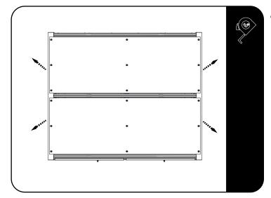
Place the Drawer System in the vehicle and center it. Making sure the Turnbuckles will all be pulling outward to the existing mounting points in the vehicle to prevent it from moving.
