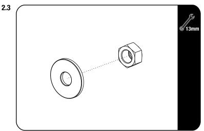
Secure the M8 x 25 x 2 Flat Washer and M8 Nyloc Nut to the pin as shown in 2.4 to secure the turnbuckles (Suplied with SSDR011).
