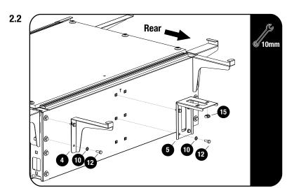
Assemble the M6 Cage Nut (Item 15) to the Rear Wing Center Plate (Item 5).
