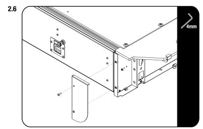
Secure the Front Face Plate LH & RH (Item 1) to the drawer system using M6 x 16 Button Head Bolts (Item 11).
