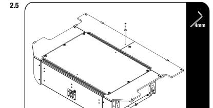
Secure the Front LH & RH Deck Set (Items 8 & 9) to the Wing Brackets.
