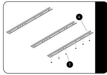
Insert six M6 Cage Nuts (2mm Material - Item 7) into the bottom of each Deck Support Channels (Item 4) as shown.
