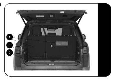
Before you start the fitment, remove the third row of seats (A), unclip the rear cargo area plastic tray (B) and the trim panel (C).
