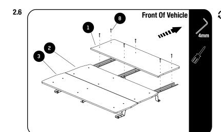
Use a suitable screwdriver to pierce the carpet over the holes in all three Decks, from the uncovered side.
