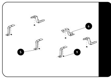
Insert a M6 Cage Nut (3mm Material - Item 9) into the bottom of each of the Mounting Brackets (Items 5 and 6) as shown.
