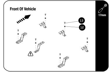
Secure the front and rear Mounting Brackets to the vehicle, using M10 x 20 Hex Bolts and M10 Flat Washers (Items 13 & 12) and fixing to OEM mounting holes.
