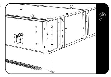
Slide two channel nuts (supplied with SSDR010 / SSW0008) into the track. Center the track under the drawer and secure with the fasteners as shown. Refer to SSDR010 / SSW0008 fitting instruction.
