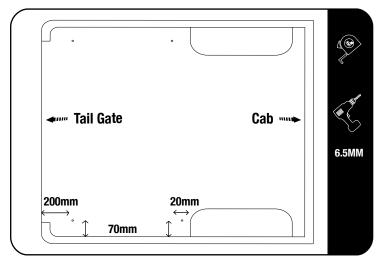
Using the measurements shown, measure and mark the positions of the holes you need to drill. Do this on both left and right sides of the load bed.
