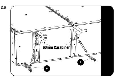
Secure the D-Rings supplied with SSDR010/SSW0008 using the holes you drilled in Step 2.1.
