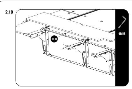
Fit the Side Decks (Items 1LH & 1RH) to the Drawer by sliding it into the C-Clips.
