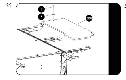
Fit the LH & RH Rear Decks (Items 2LH & 2RH) with M6 x 30 Countersink Screws and M6 Finishing Washers (Items 7 & 8) as shown.
