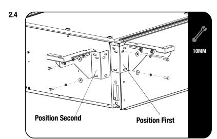
When fitting the Rear Corner Wing Brackets take note of the position.
