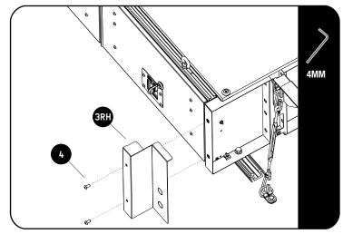
Secure the Front Faces (Item 3LH & 3RH) to the Cage Nuts in the Drawer System (SSDR010) using M6 x 12 Button Heads (Item 4) as shown.
