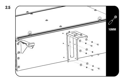
The Rear Support Bracket is also part of SSWS001. Fit and secure with the fasteners supplied with SSWS001 as shown.
